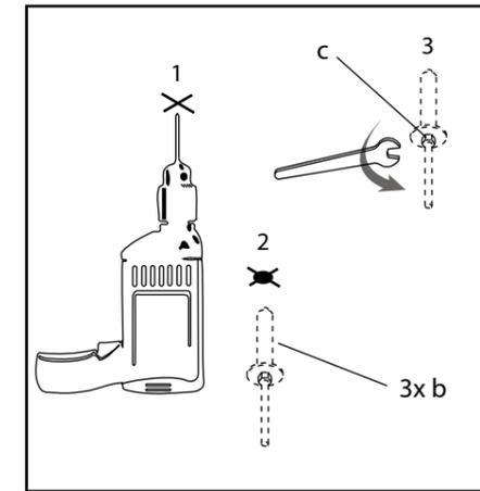
Drill in the marked points. Insert the 3 rawplug fixings not provided (b) and fix them by tightening the nut (c).
