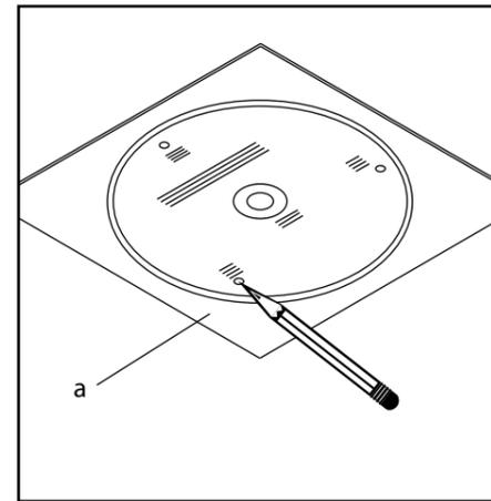
Mark the drilling points by using the cardboard template (a) contained in the package.
