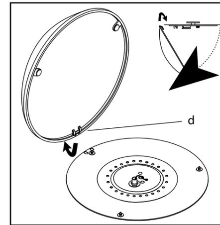
Remove the diffuser by turning it around the hinge (d).
