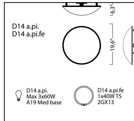
Wall or ceiling lamp for incandescent or fluorescent bulbs. Thermoformed reflector of silkscreened polycarbonate with weft drawing, easily removable for maintenance. Metal parts of anodized aluminium.
