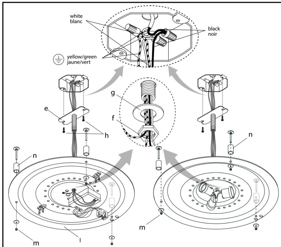
Disassemble the "Cross bar" (e) by unscrewing the nut (f). Make the electrical connections in the "Junction Box" noting Live and Neutral (L- N). Fix the "Cross bar" to the "Junction box" using screws (h), which are not supplied. After fixing the plate (l) to the "Cross bar" using the nut (f) and washer (g), place the spacer (n) and screw the nuts (m) and washers to the plugs.
