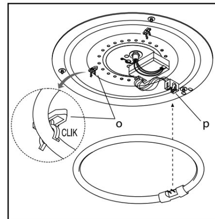
Insert the lamp in the lamp-holder (p) by releasing the sealing spring (o).
