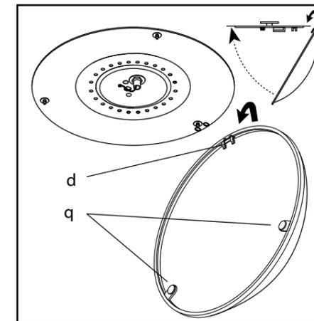
Mount the diffuser by inserting the hinge (d) into the 2 slots on the plate and rotate it until the two magnets (q) attach.
